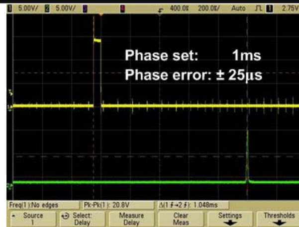
Phase control on the chopper mock-up machine
